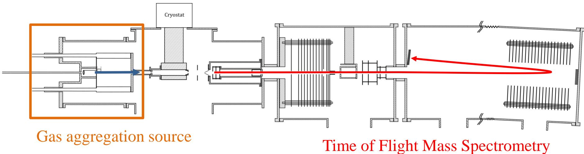
Experimental setup designed to perform collisions between mass selected clusters and atomic or molecular vapor (attachment cross-section, fragmentation cross-section, nanocalorimetry, spontaneous thermal evaporation, ...).
