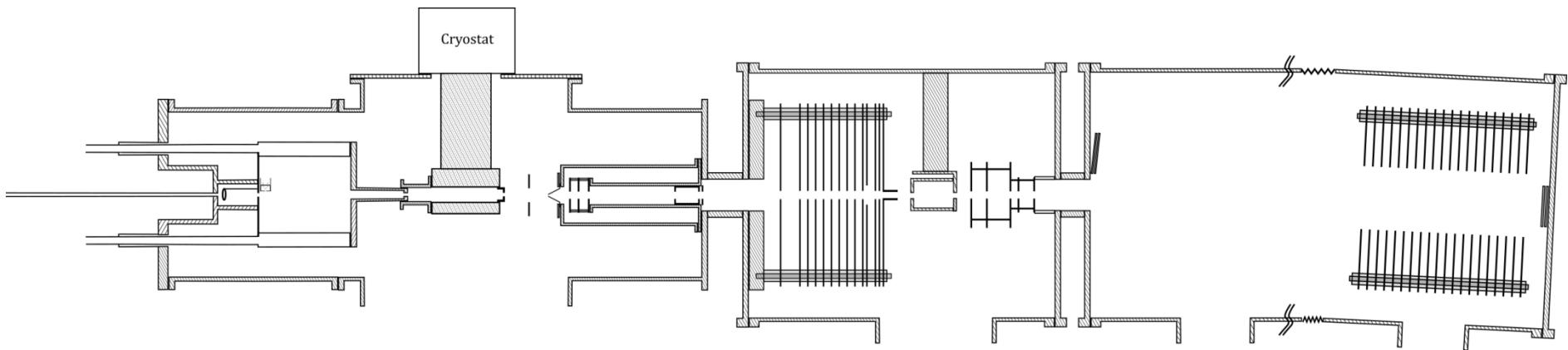
Experimental setup designed to perform collisions between mass selected clusters and atomic or molecular vapor (attachment cross-section, fragmentation cross-section, nanocalorimetry, spontaneous thermal evaporation, ...).
