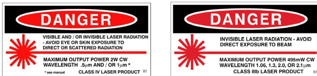
Warning Labels - Located on top of the laser head.
