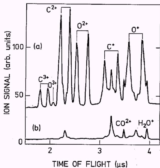
FIG. 2. TOF ion mass spectra of CO with the laser polarization (a) parallel to the drift tube axis and (b) perpendicular to the drift tube axis. The scale for the ion signals is the same for both spectra.
