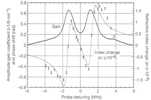
**Figure 3** Measured refractive index and gain coefficient. The superimposed curve over the index data is obtained using equation (1) with parameters  $v_1$ ,  $v_2$  and  $\gamma$  obtained experimentally.
