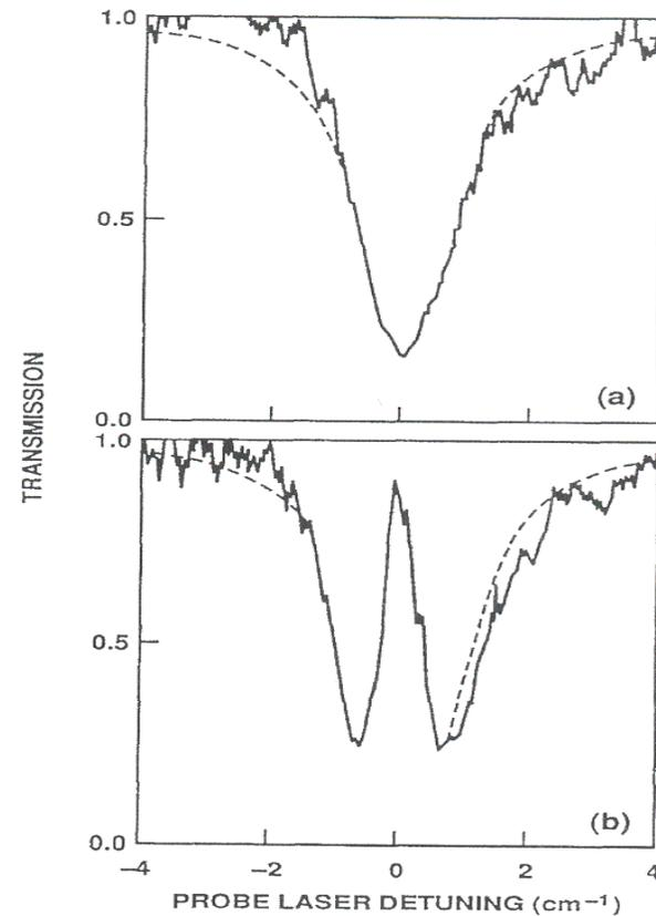
FIG. 2. Transmission vs probe laser detuning for (a)  $\Omega_{23} = 0$  and (b)  $\Omega_{23} = 1.3 \text{ cm}^{-1}$ ,  $\Delta\omega_c = -0.2 \text{ cm}^{-1}$ . Minimum transmission is  $\exp(-1.7)$ .
